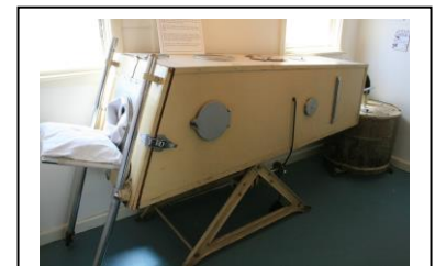
Fig. 2: The Both cabinet respirator was built of plywood, an order of magnitude cheaper, easy to manufacture, and lighter than previous devices. Note air pump at right, and the pivot point on the support legs that allows patient angle to be adjusted to drain fluid from the lungs.
