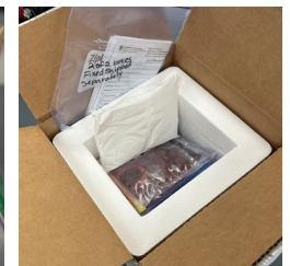
Well-packaged: leak proof inner and outer containers; labeled specimens in their own containers and bags; submission form in separate bag.
